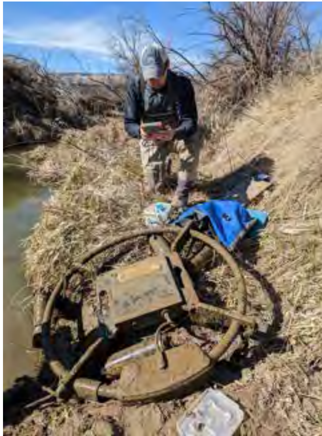
Figure 2. Photograph of a 3-foot diameter submersible PIT tag antenna. The circular tubing has a small copper wire inside of it which produces a low frequency electromagnetic field. When this field is disturbed by a PIT tag, the tag's unique alpha-numeric code is read and saved, along with the date and time of the detection by the datalogger on the antenna.
